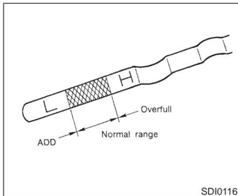
● It is normal to add some oil between oil maintenance intervals or during the break-in period, depending on the severity of operating conditions.
