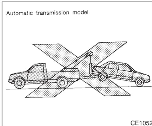
Towing an automatic transmission model with rear wheels raised (with front wheels on the ground)
