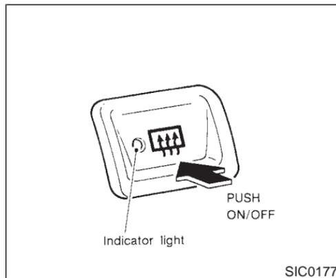
To defog the rear window glass and outside mirrors, start the engine and push the switch on. (The indicator light will come on.) Push the switch again to turn the defogger off.
