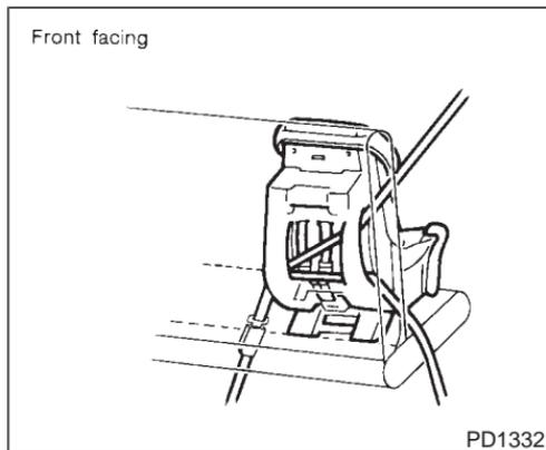
seat belt is allowed to wind back into the retractor, the automatic locking mode (child restraint mode) is canceled; the seat belt may be used as normal and will only lock during a sudden stop or impact.
