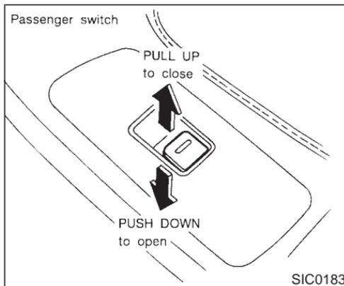
The passenger side switch will open or close only the corresponding window. To open or close the window, hold the switch down or up.
