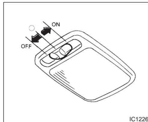
The interior light has a three-position switch. When the switch is in the center "○" position, the light will illuminate when a door is opened.
