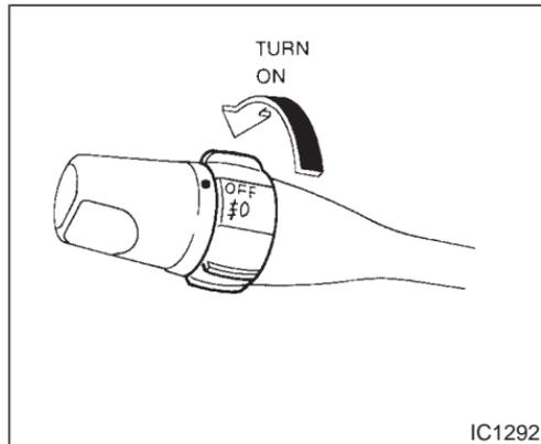
To turn the fog lights on, turn the headlight switch to the “
