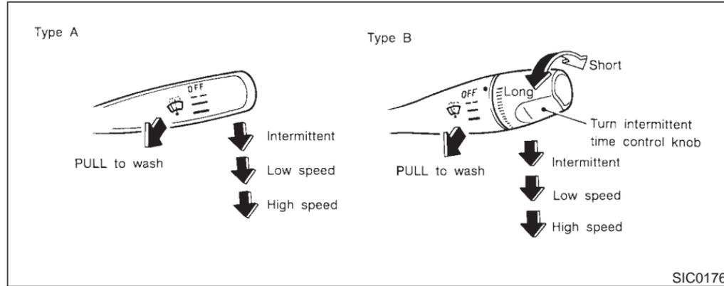
The windshield wiper and washer operates when the ignition key is in the "ACC" or "ON" position.
