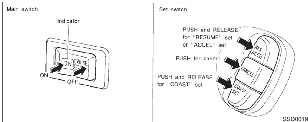
The cruise control allows driving at a speed between 30 to 89 MPH (48 to 144 km/h) without keeping your foot on the accelerator pedal.
