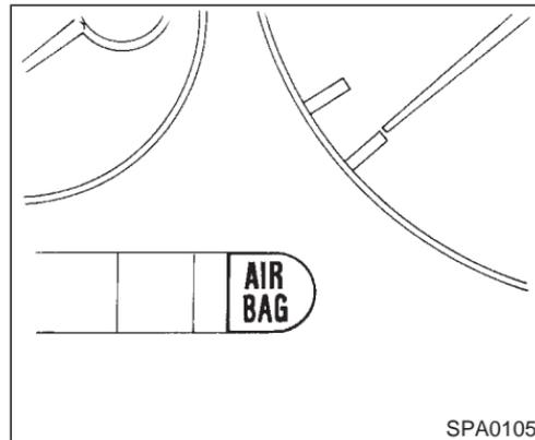
The air bag light, displaying "AIR BAG" in the instrument panel, monitors the circuits of the air bag. The circuits monitored by the air bag light are the diagnosis sensor unit, air bag modules and all related wiring.
