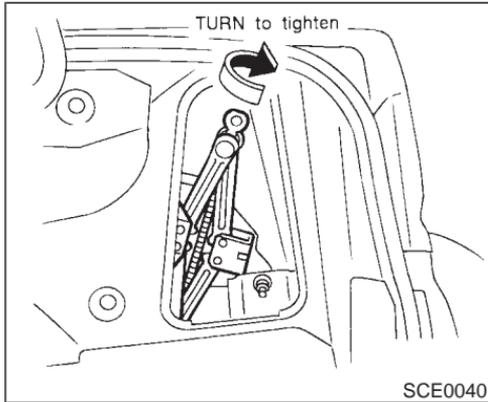
5. Securely store the spare tire and jacking equipment in the vehicle.
