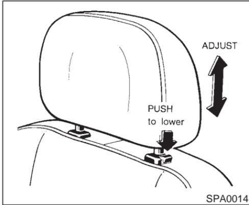
lower, push the lock knob and push the head restraint down.
