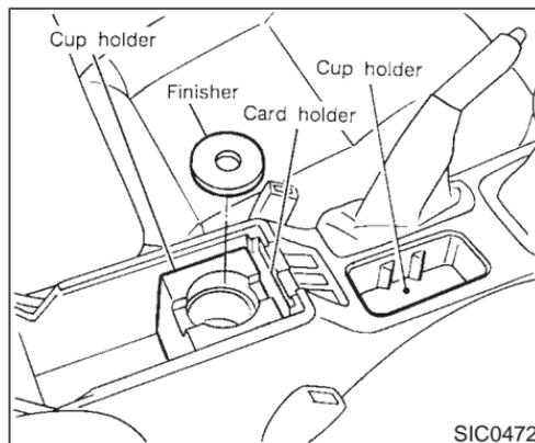
To accommodate different sized cups, remove the finisher.
