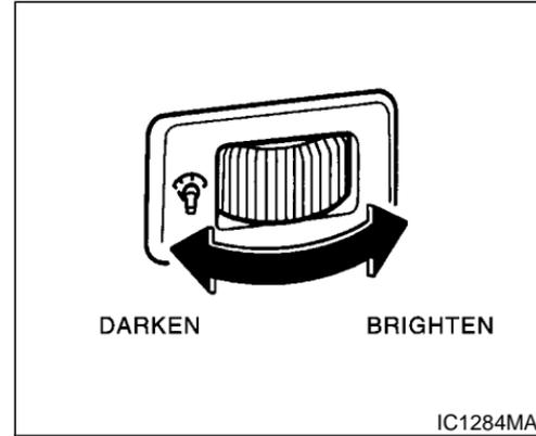
The instrument brightness control operates when the light switch is in the "☰" or "☷" position.
